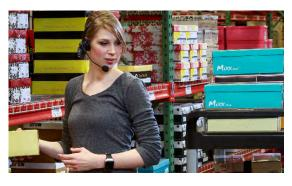
items he picks, reducing pick quantity errors. And to eliminate mistakes due to confusion over unit of measure or pack factors, users can be required to speak the pack type (each, bottle, case, inner pack, etc.) of items as they are picked.
